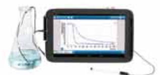
Tethered active or capacitive stylus and plug-in temperature probe
